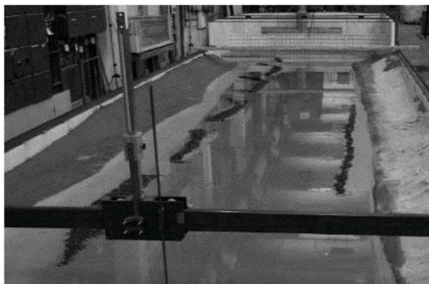
Figure 4. Physical model of the pilot section for optimising the longitudinal training dams (LTDs).
